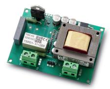
The TSR01 is an electronic relay for the switching of transformators. It switches one or more single phase transformers, either from an idle state or loaded state without inrush current. By our smooth switching procedure the inrush current is eliminated, not only reduced.
